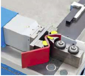
Bending tool 30° with U shaped die for bending flat bars up to 30°. Max. 16 x 200 mm.
