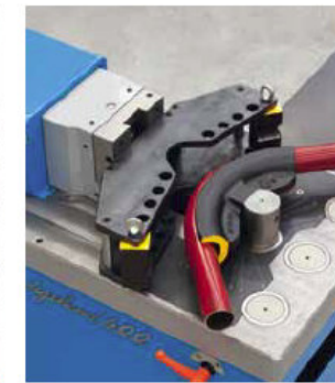
2 jaw bending tool for thick wall pipes from 3/8" gas (17.2 mm) up to 2" gas (60.3 mm) and round bars, up to 90°.
