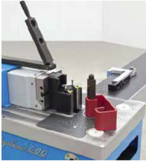
Bending tool with pin Ø 50 mm, H=200 mm, revolving pin single V die and antiflection bar. max. 200 x 8 mm. Patent Pending.
