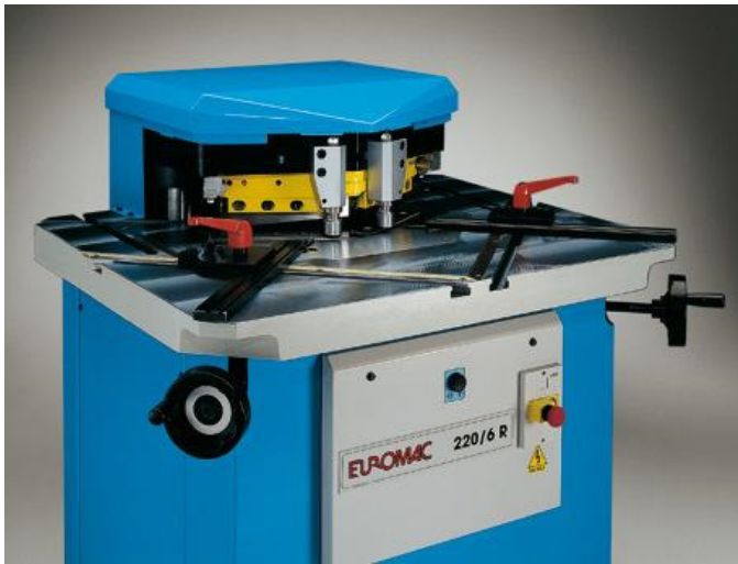
Variable Angle Notching Infinitely adjustable from 30° to 140°. (variable angle models only)
